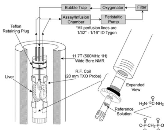
**Figure 1.** Essential components of the perfused liver apparatus. Inflow of perfusion buffer is via the portal vein cannula. The expanded view of the bottom of the NMR tube on the right shows an external reference solution which may be used for absolute quantitation.
