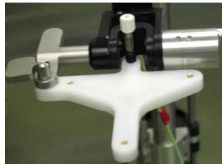
Fig. 2 Specially designed hand piece of optical tracking system attached to the end effector.
