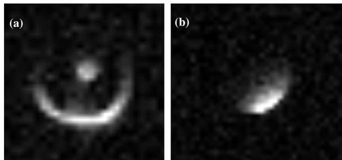
Figure 3. HP  $^{129}\text{Xe}$  images of the (a) storage and (b) delivery chambers. Experimental parameters: 64X64, FOV 12.0/12.0 cm, Flip angle: 4°, TR = 25 ms, TE = 3.4 ms, and numbers of repetition: 40.
