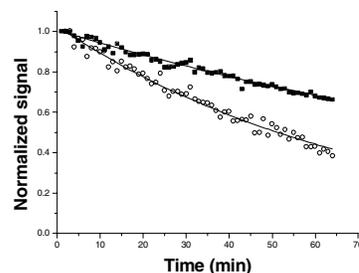
Figure 2.  $T_1$  signal decays of HP  $^{129}\text{Xe}$  gas in the storage (■) and delivery (○) chambers. Measurements were carried out with 64 accumulated scans of a ca. 4° hard pulse with a repetition time of 60 sec.
