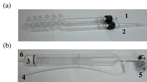
Figure 1. Pictures of the home-designed storage/delivery system, (a) spiral storage chamber, and (b) delivery chamber, consists of inlet valve (1, 4), outlet valve (2), Teflon piston (3), pneumatic valve (5), and external pressurization air inlet (6).
