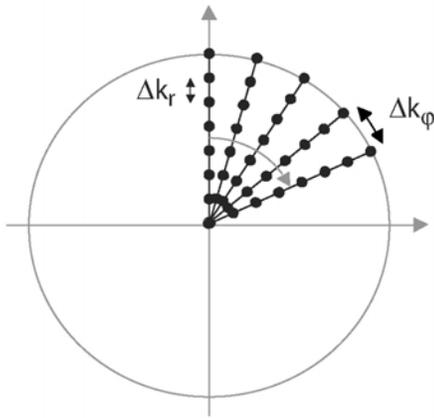
**Fig 1.** Schematic k-space trajectory of the radial in-plane readout pattern.
