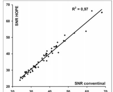
Fig. 2: Quantitative analysis results from 6 healthy volunteers. SNR of HoPE is plotted against SNR of conventional imaging. Values correlate with a high coefficient  $R^2=0.97$ .
