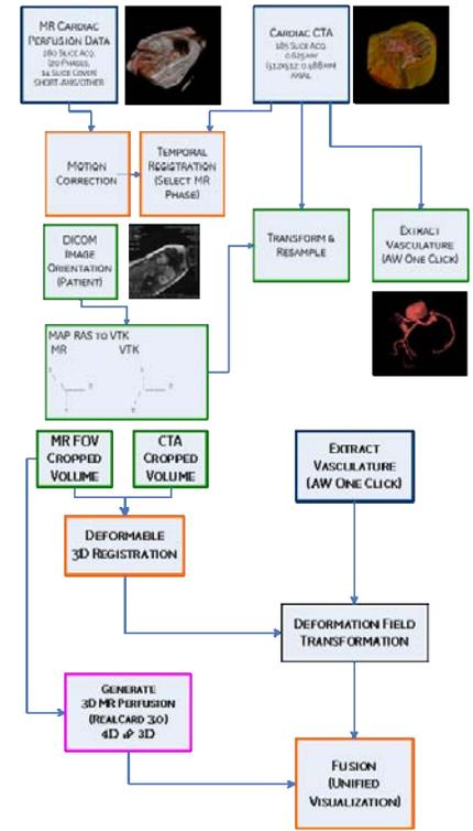
Figure 1: Flowchart illustrating the Cardiac MR-CT Fusion Pipeline.
