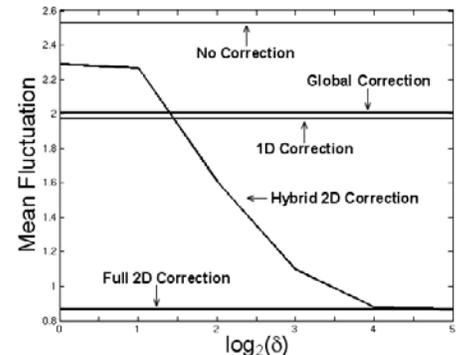
Figure 2: Mean percentage noise fluctuation within the gray matter ROI (acquired using a 2-shot EPI sequence) with hybrid 2D navigator echo correction for  $\delta = 1, 2, 4, 8, 16,$  and  $32$ . The mean noise fluctuation with no correction, global correction, 1D correction, and full 2D correction are shown for comparison. When  $\delta = 16$ , the performance of hybrid 2D correction is virtually identical to full 2D correction.
