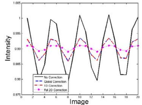
Figure 1: Normalized peak-to-peak pixel intensity fluctuation for an ROI with no navigator echo correction (2.22%), global correction (0.759%), 1D correction (0.752%), and full 2D correction (0.199%). Full 2D correction reduced this noise by an additional 0.55% beyond global or 1D correction.
