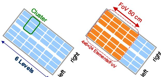
Figure 1: The PA Matrix consists of 36 elements, organized in 6 levels with 2 clusters per level. A total of 24 PA Matrix coil elements, or a total of 4 levels in z, are sufficient to cover a FoV of 50cm.
