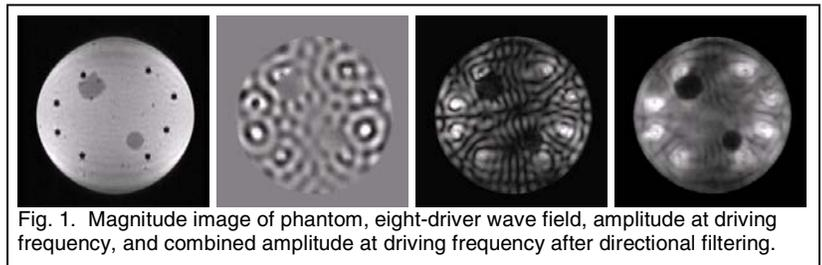
Fig. 1. Magnitude image of phantom, eight-driver wave field, amplitude at driving frequency, and combined amplitude at driving frequency after directional filtering.
