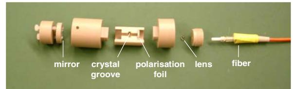
Fig. 1: Exploded view of the reflection mode Faraday position sensor
