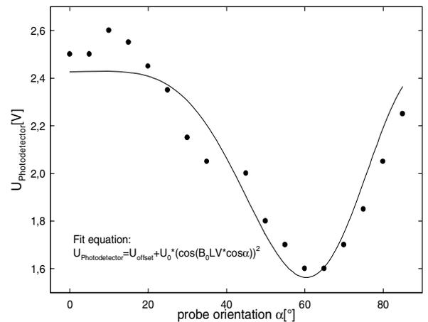
Fig. 2: Photo-detector voltage at different sensor-orientation angles towards  $B_0$
