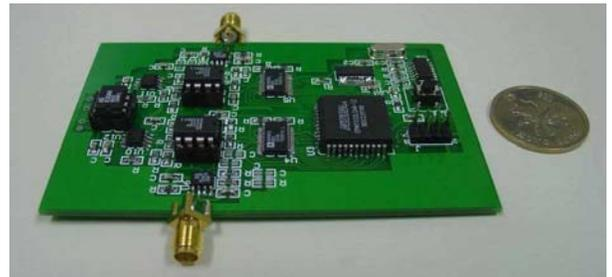
Fig. 2 MRI two channel FDM PCB prototype
