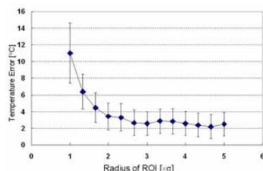
Figure 1. Relationship between the radius of ROI and the temperature estimation error near the sonication center. The values are the mean for the 10 different sonication locations. The error bars denote the ranges of the standard deviations.
