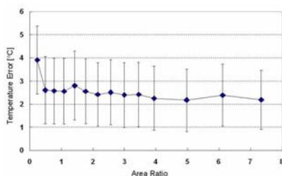
Figure 2. Temperature estimation error as a function of the area ratio between RFE and ROI. The mean and the standard deviations for the 10 sonication locations are shown.
