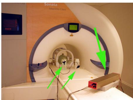
**Fig. 1:** Camera system (thick arrow) and LED probes (small arrows) of the optical tracking device.
