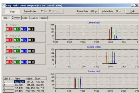
**Fig. 2:** Position in pixel units of individual LEDs (different colors) as seen by the three CCD elements of the active optical tracking device.
