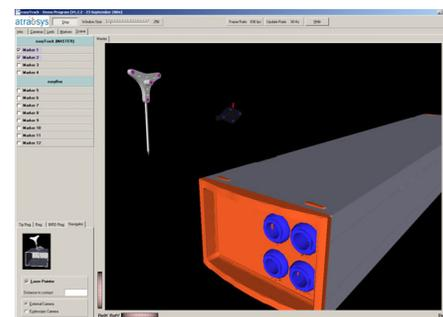
**Fig. 3:** Screenshot of the atrac software showing a 3D representation of the easyTrack and the markers.
