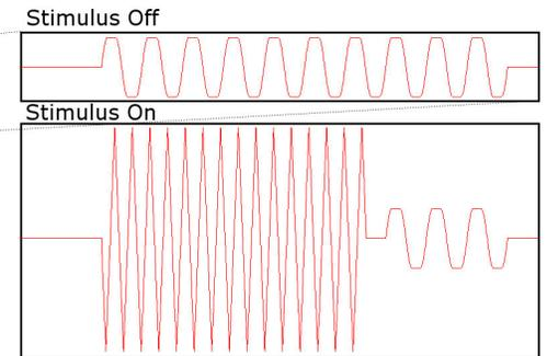
Fig. 1b: Enlarged plot of the additional block of x-gradients in figure 1a (“stimulus off”). For the stimulation periods (“stimulus on”), it is exchanged for a 15ms pulse of 1-kHz triangular gradients of maximum amplitude. To avoid eddy current induced artifacts, the last 7ms of both gradient patterns are identical.
