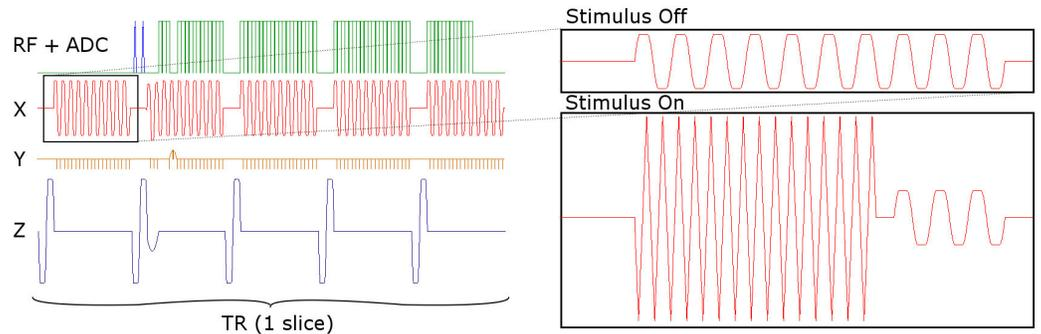
Fig. 1a: LINA-EPI sequence timing diagram for the acquisition of a single slice. The black frame indicates the additional gradients which here (for “stimulus off” case) serve to continue the unpulsed gradient sound of the sequence.
