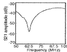
Fig 1: S21 between direct neighbors in a loaded PSA
