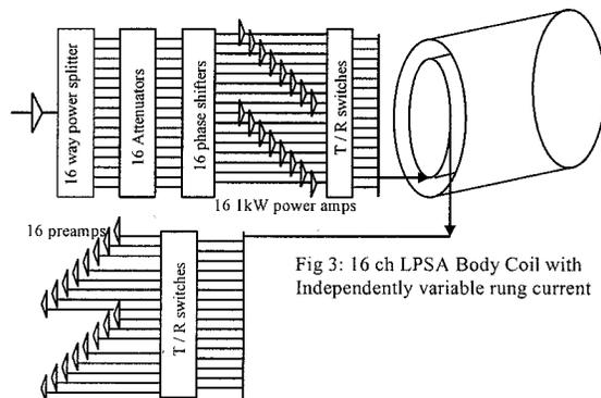
Fig 3: 16 ch LPSA Body Coil with Independently variable rung current
