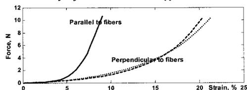
Figure 1: Mechanical strain measure of meat phantom.
