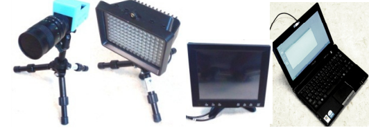
Fig.1. Optical tracking camera, IR illuminator, monitor and recording palmtop located outside of magnet bore.
