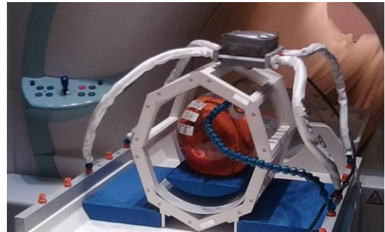
Figure 1: Photograph of the tracking camera setup above the head coil.
