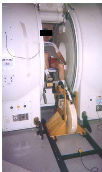
Figure 1. 59-year-old subject pedaling a custom MR-compatible stationary cycle in the GE 0.5T open magnet
