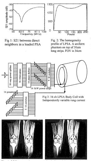
Fig 4: LPSA array images, regular(left) and SENSE with R=2 (right). FGRE, TR=150ms, TE=3.3ms, 7mm slice, FOV 48 cm
