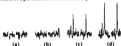
Fig. 2 ^{17}\text{O} spectra acquired using the implanted vessel coil: (a) empty coil, (b) coil wrapped by a chamber filled with natural abundance \text{H}_2\text{O} , (c) a glass capillary (o.d.=1.46mm, i.d.=0.66mm) filled with natural abundance \text{H}_2\text{O} , and (d) in vivo blood in the rat carotid artery of natural abundance.
